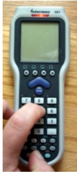
3. While holding 5, press and release power button.
