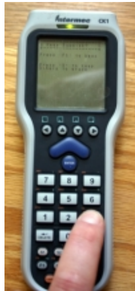
8. At "Keep RAM Disk?", press F1, then press 3. (After a pause, CK1 will flash blue.)
